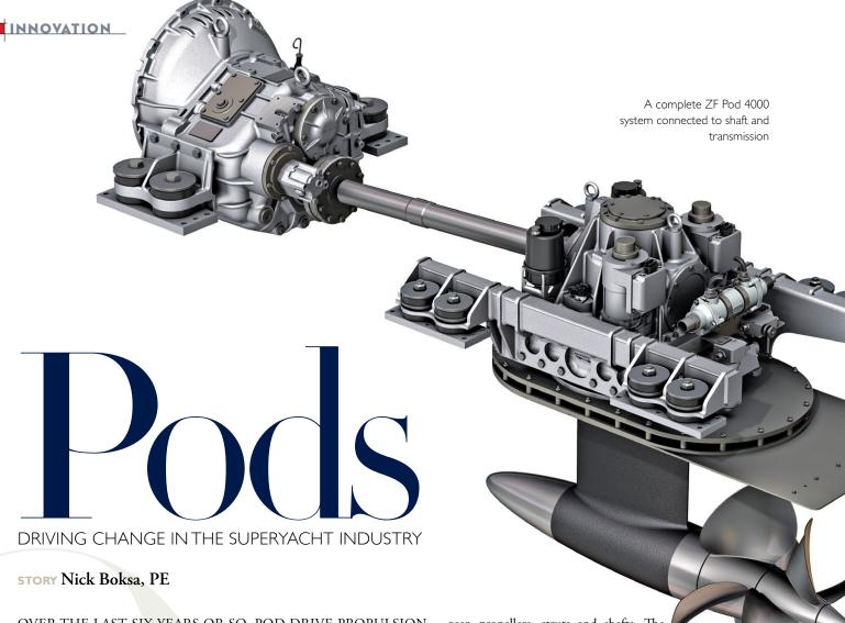
OVER THE LAST SIX YEARS OR SO, POD DRIVE PROPULSION has become an exciting option for owners, builders and designers seeking more efficient ways to power their yachts. The benefits of pod drives—maneuverability, operational efficiency and design flexibility—have proven irresistible within the industry.
