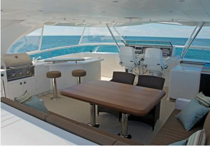
**ABOVE:** In the open flybridge version, the PC58 can be equipped with a removable windscreen ensuring guests enjoy the flybridge's amenities, including a wet bar and grill, in any kind of weather; the helm console features easy-to-read monitors by Garmin, a stainless-steel wheel and a ZF joystick
